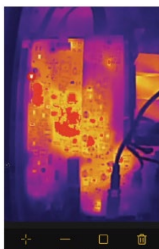
Over-temperature area alarm
