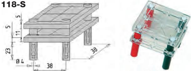
Component-holders, pitch of 19 mm, screw connection - 20 A, < 33 V AC < 70 V DC
