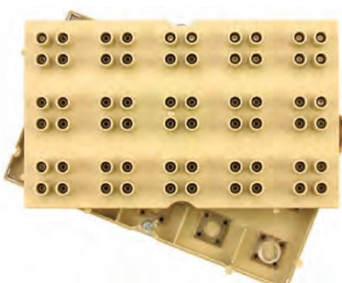
2 pole component holder, very robust type, connection by  $\varnothing$  4 mm plugs, many contacts, 38 mm pitch, insulator + transparent cover easy for silk-screen printing.
