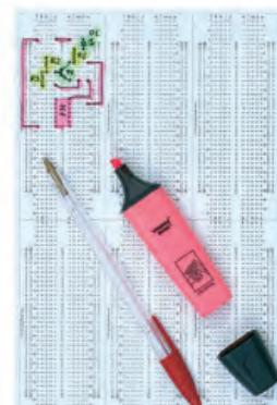
**CIRCUIT TEST PANELS** Circuit boards without solder
