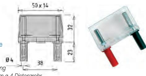
4 pole component holder (of course usable for 3 poles) very robust type connection by  $\varnothing$  4 mm plugs, many contacts pitch of 38 mm.
