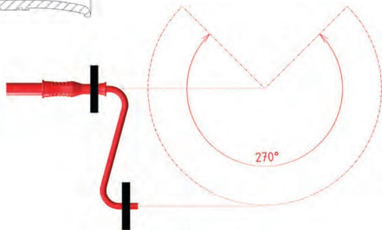
2 - Rotational flexing test : 2 x 250 270° flexings (crank style movement).
