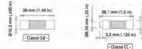
Material : Contacts : brass and CuBe/Ni (Au/Ni feasible). Insulators : Polyamide and Polypropylene.
