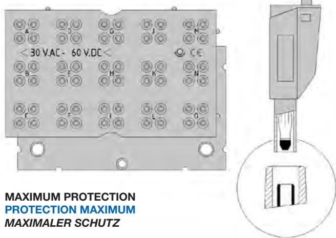
With a very robust conception, this all directions modular basic plate presents the following characteristics : 15 poles with a pitch of 38 mm. Each pole is composed of a connector and 4 protected  $\varnothing$  4 mm sockets with a pitch of 19 mm and alphabetical labels which allow many possibilities.
