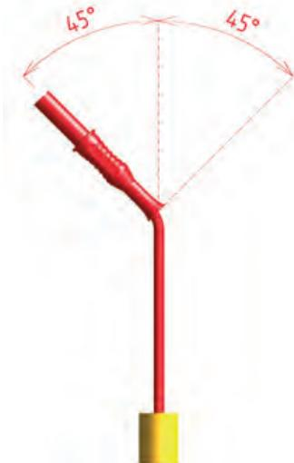
1 - Flexing / Pull test : 2 x 5000 90° flexings with a 20 N pull force (windscreen wiper style movement).
