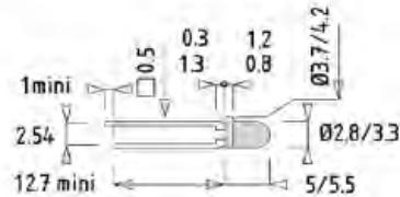
Led ø 5 mm, standard brightness, 60°, 2.54 mm pitch
